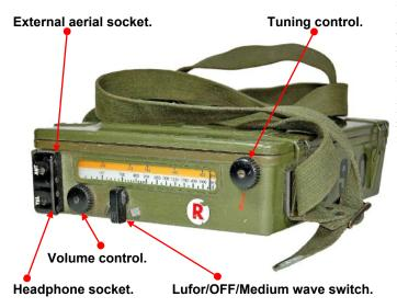
Front panel view of Mt 910 B LUFOR receiver.
